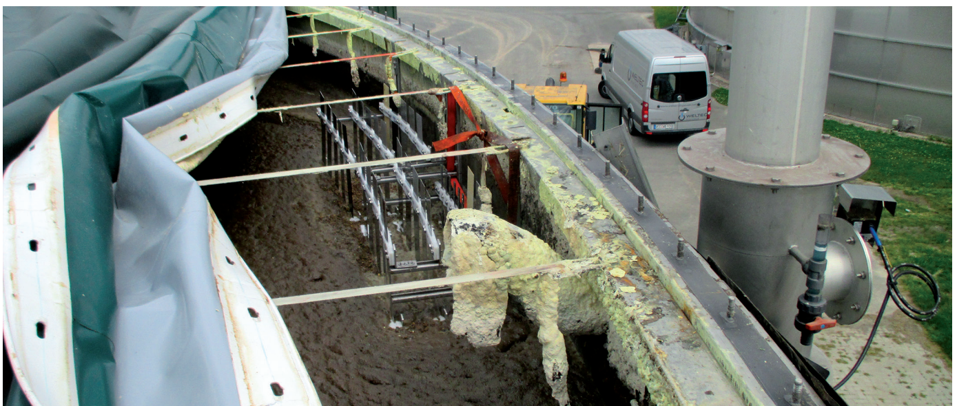
Figure 8 Stainless steel specimens inside the German biodigester
