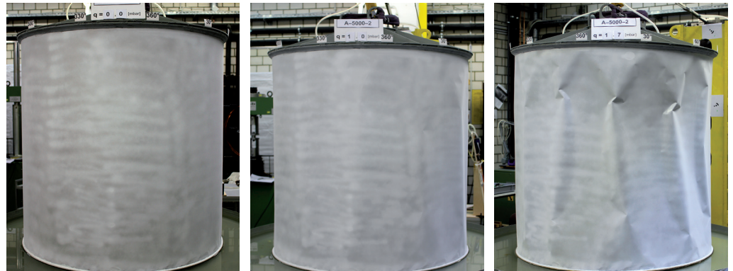
Figure 12 Austenitic stainless steel shell under reducing internal pressure
