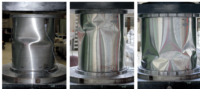
Figure 11 Buckling patterns in duplex shells subject to axial loading Left: r/t = 50 Middle: r/t = 150 Right: r/t = 333
