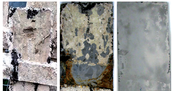
Figure 9 Sample 1.4509/2B after exposure for 6 months in a biodigester
